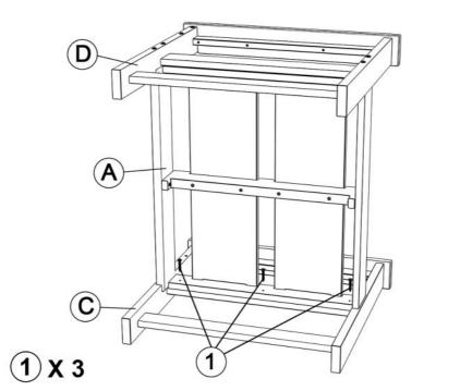
· As shown in the figure, Fix A and C with 1
