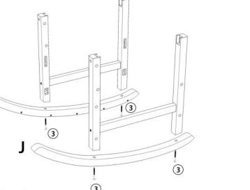
Attach "(I)" and "(J)" to the Legs - Using "3 M6
