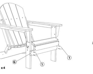
Attach "Back Stretcher (H)" to "Chair Seat Frame (A)" - Using "5 M6 × 35MM Bolts", tighten with hex key.
