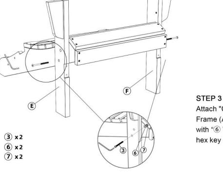
Attach "Chair Legs (E/F)" to "Chair Seat Frame (A)" - Using "3 M6 × 60MM Bolts" with "6 Washer" and "7 Nut", tighten with hex key and wrench.
